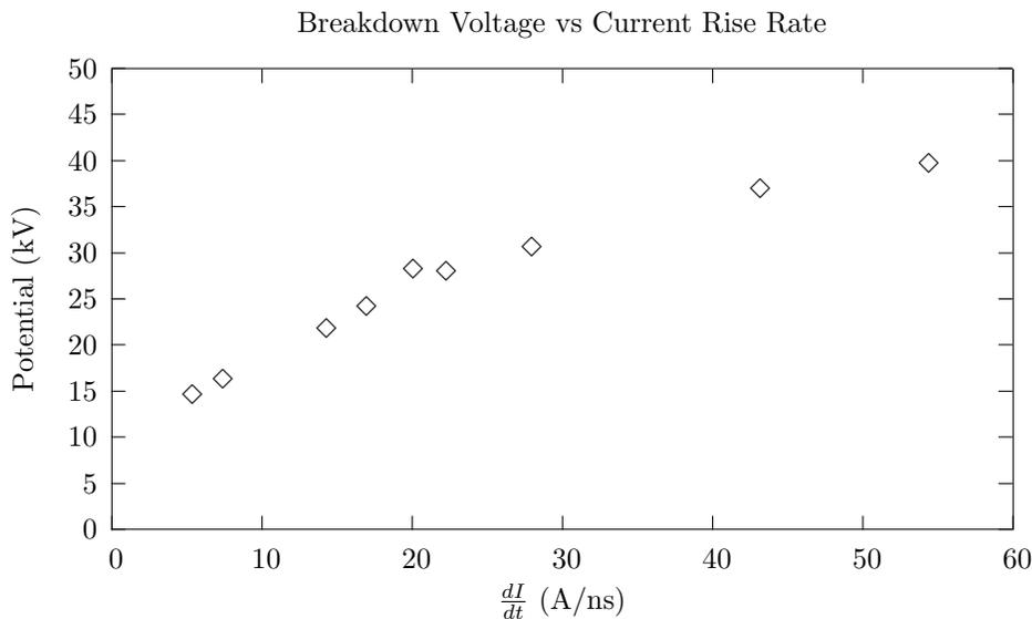
Figure 4: Breakdown voltage as a function of  $\frac{dI}{dt}$  for shot 3 cm, 25  $\mu\text{m}$  copper wires.
