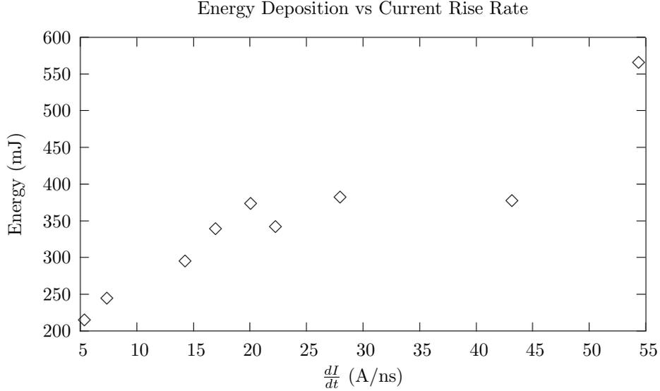
Figure 3: Energy deposition as a function of  $\frac{dI}{dt}$  for shot 3 cm, 25  $\mu\text{m}$  copper wires.
