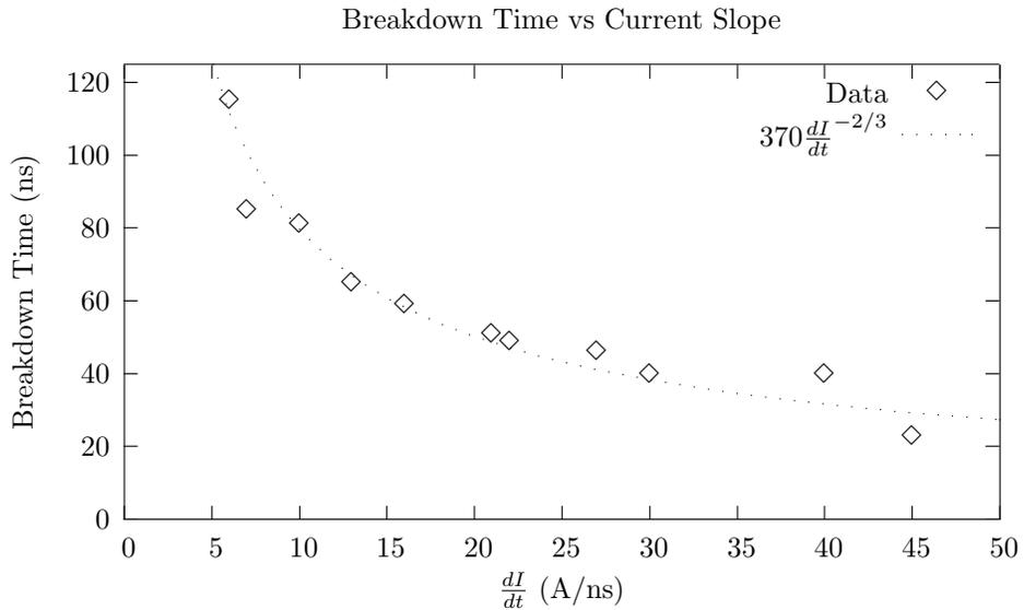
Figure 2: Wire data demonstrates behavior similar to that predicted for transverse effect plasma
